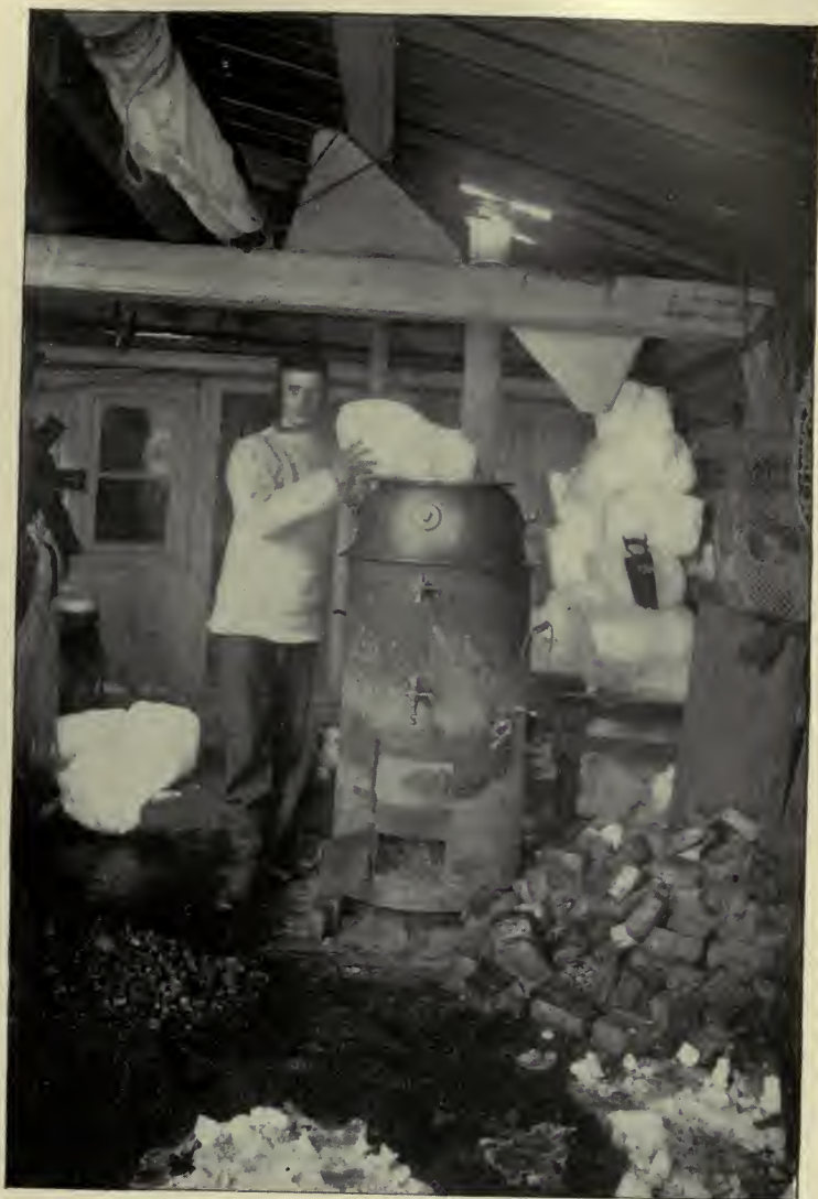
M. van Rysselberghe at the condenser, which was converted into a snow melter. This apparatus, by the combined ingenuity of van Rysselberghe and van Mirlo, was taken out of the engine-room, placed on deck, and so altered that it burned seal blubber. From this the Belgica was supplied with water,
