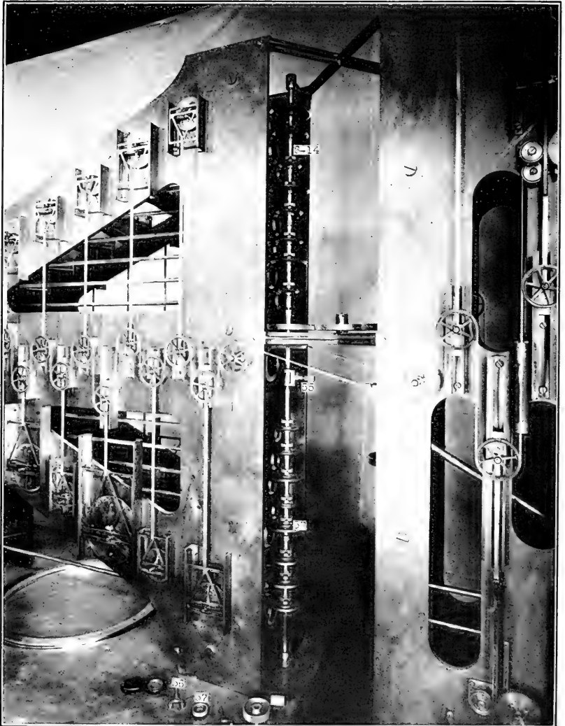
Fig. 19.—FORWARD DRIVING SHAFT, REAR COMPONENT SECTION, TIDE-PREDICTING MACHINE.
