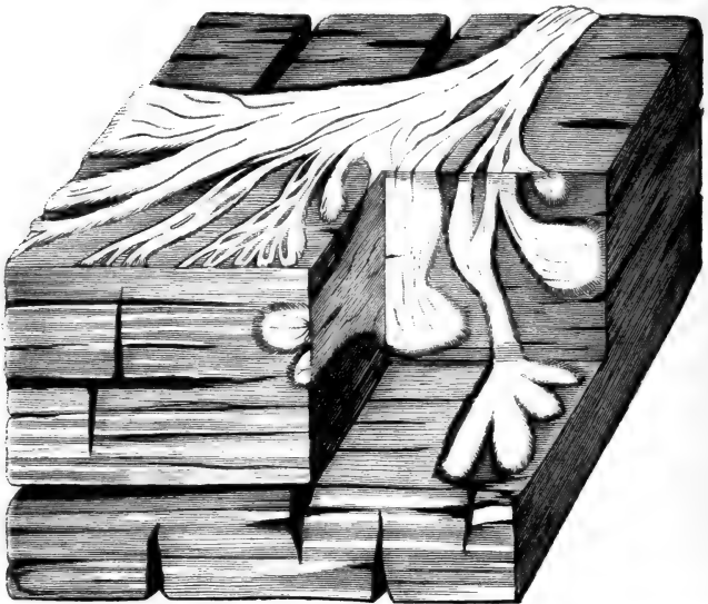
FIG. 24.—A piece of pine-wood attacked by the mycelium of Polyporus vaporarius . The timber has warped and cracked under the action of the fungus, becoming of a warm brown colour at the same time; in the crevices the white strands of felt-like mycelium have then increased, and on splitting the diseased timber they are found creeping and applying themselves to all the surfaces. Except that the colour is snowy white, instead of gray, this mycelium may easily be mistaken for that of Merulius . The fructification which it develops is, however, very different. (After R. Hartig.)
