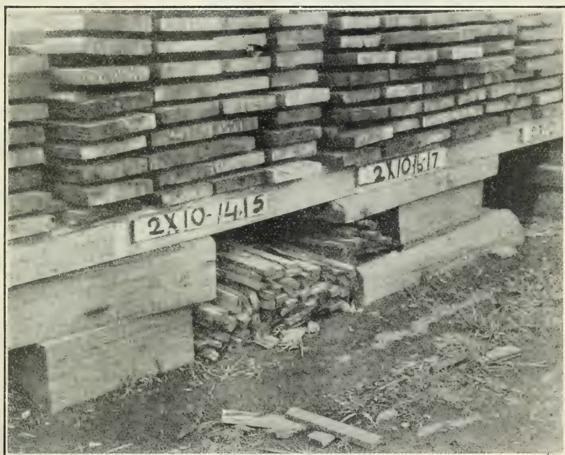
FIG. 25.—Piling sticks placed on wet ground beneath the skids. In order to keep them free from infection, such sticks should never be placed in contact with the soil.
