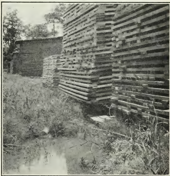
FIG. 4.—Lumber piled on low swampy land at a Texas sawmill. The serious decay in this yard is due to the excess of soil moisture and poor circulation beneath the stacks.
