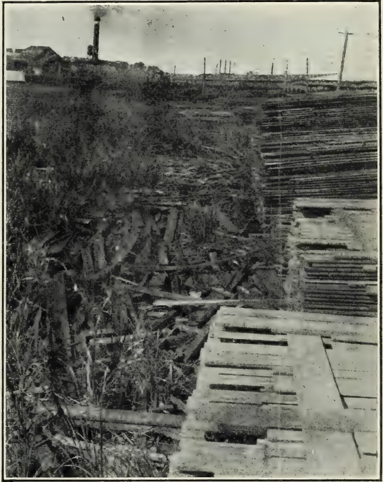
FIG. 9.—Pine and hardwood lumber which has rotted in storage in the yard shown in figure 11. Instead of burning the débris it was thrown into an adjoining rice swamp. Fungi developing on this débris will again infect the sound lumber.
