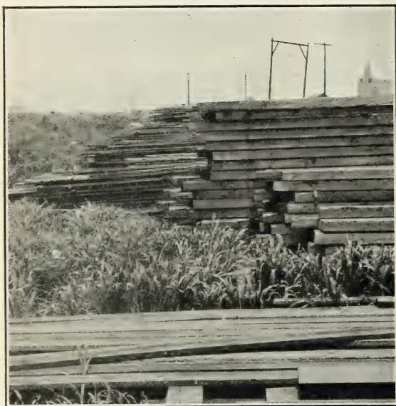
FIG. 5.—Pine lumber piled in a swamp on high skids over standing water at New Orleans, La. Note the luxuriant vegetation, which checks proper air circulation beneath the piles.
