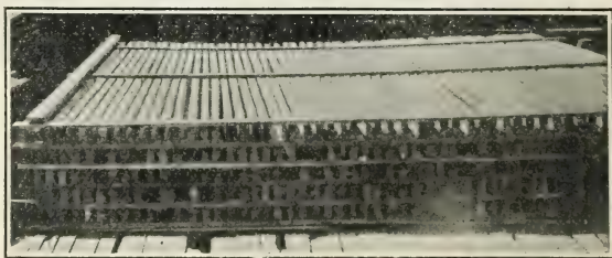
FIG. 27.—Edge-piled 2 by 4 pine at an Arkansas mill. This method of piling permits better vertical air circulation and consequently more rapid drying and less danger from decay during storage.
