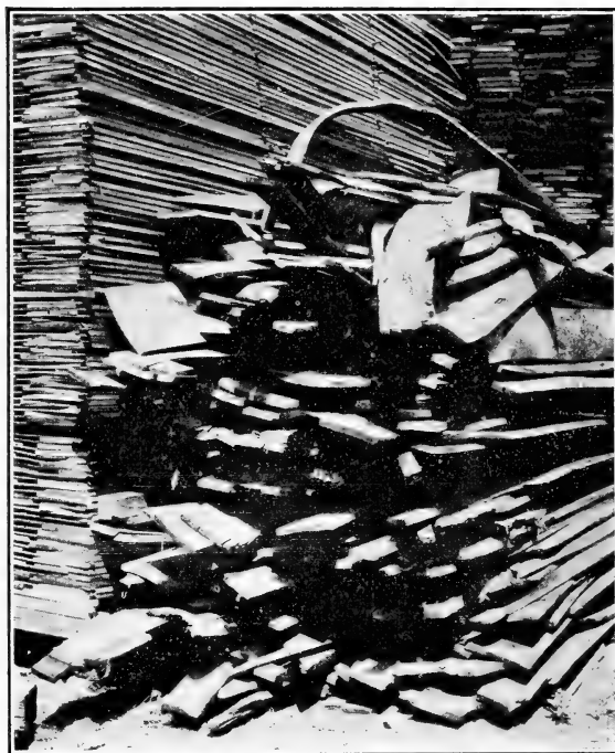
FIG. 10.—Partially rotted hardwood boards piled against a lumber stack. Infection will spread by contact to the sound lumber.
