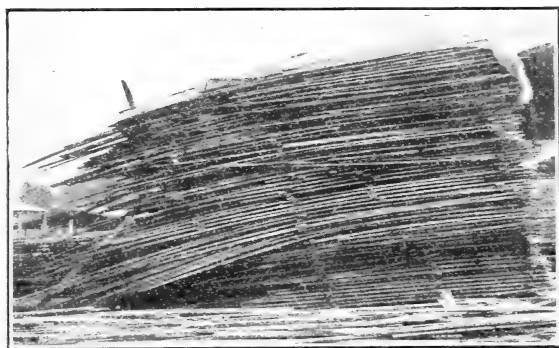
FIG. 29.—A stack of pine lumber of uneven lengths. Note the irregular distribution of the piling sticks and the consequent warping and twisting of the boards.
