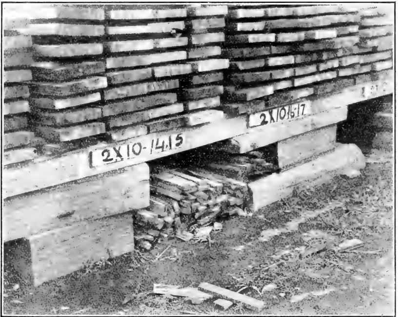
FIG. 25.—Piling sticks placed on wet ground beneath the skids. In order to keep them free from infection, such sticks should never be placed in contact with the soil.
