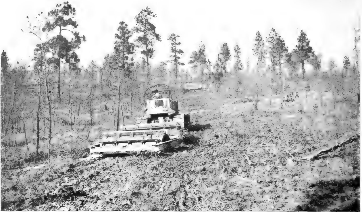
FIGURE 62. — Mechanical destruction of scrub oak is one way to prepare the site for regeneration in the Sandhills.
