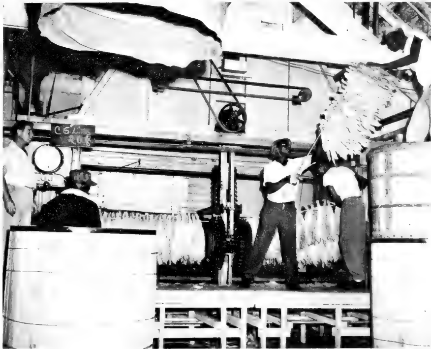
Figure 37.--Flue-cured tobacco being placed into hogs-heads as it comes from the redrying machine.
