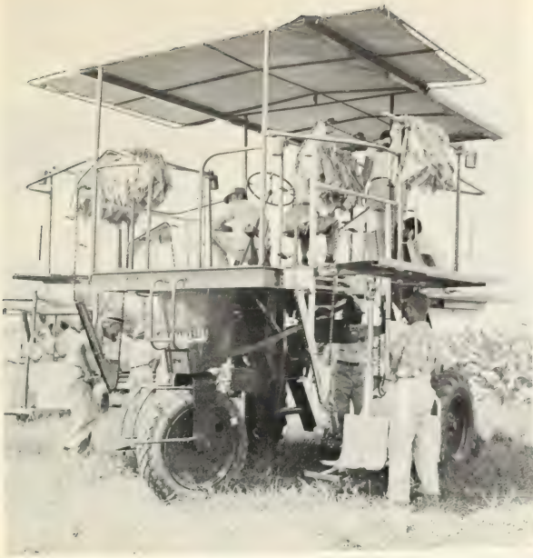
Figure 8.--A self-propelled priming platform of a type widely used in flue-cured areas.
