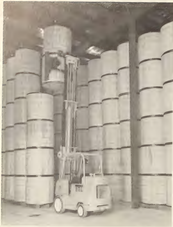
Figure 39.--This new method of storing hogsheads saves labor and increases warehouse capacity.
