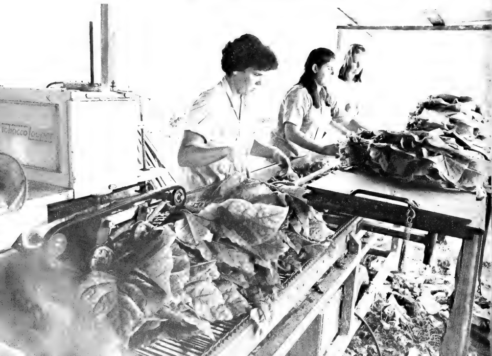
Figure 11.--This "tying machine" uses twine to secure flue-cured leaves to sticks for banging in the curing barns.
