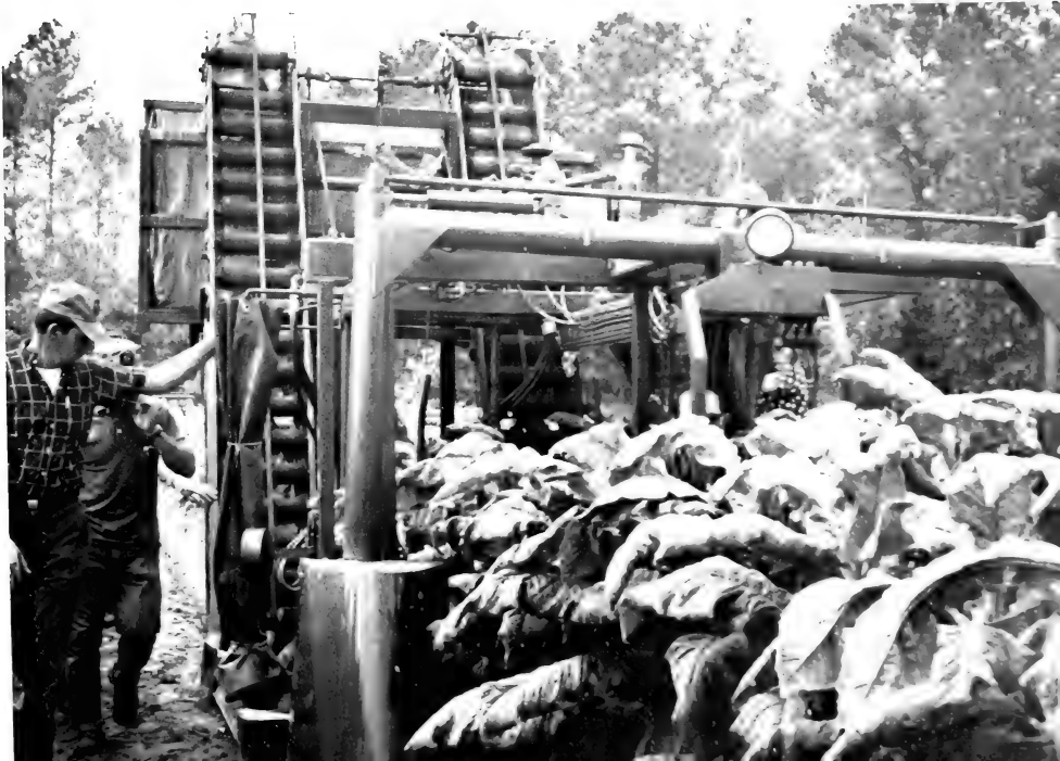
Figure 9.--Experimental version of mechanical barvester developed for flue-cured tobacco.
