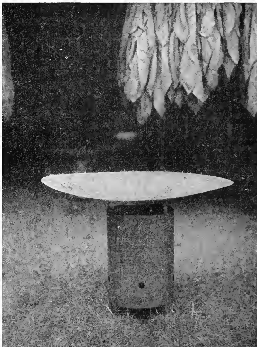
* FIGURE 38. Salamander and spreader designed for use in tobacco sheds. Note that 18-inch height permits spread of heat underneath lower tier of tobacco.
