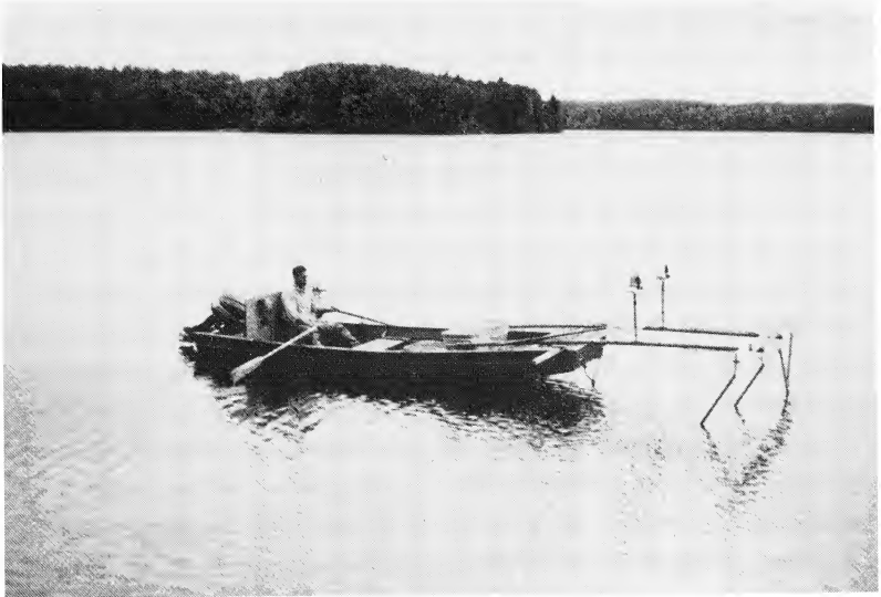
Fig. 23. William Helm and Wisconsin's first operational boom shocker, 1958. The shocker was built by Helm and was used for his walleye studies on Little John, Erickson, and Sparkling Lakes in northcentral Wisconsin. Source: William Helm.
