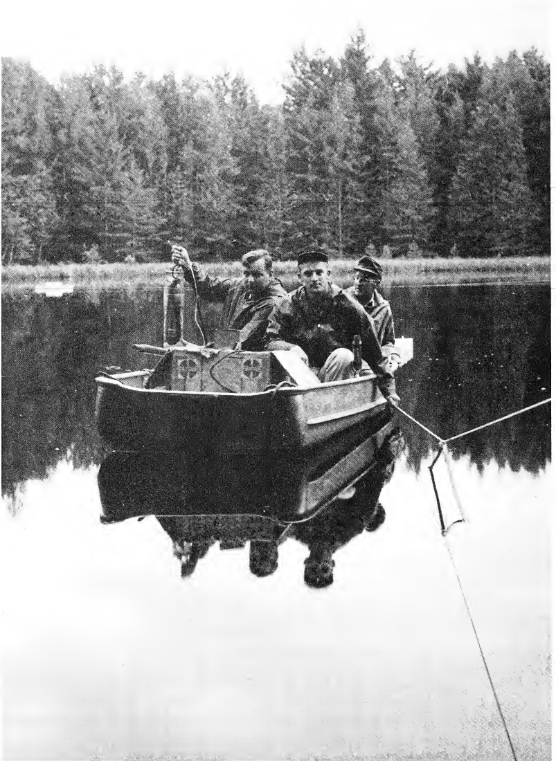
Fig. 24. Physicist John W. Anderegg, Gene Likens, and A. D. Hasler on Cather Lake in northern Wisconsin about 1961. Anderegg is holding a scintillation counter used for the detection of isotopes in a study of the movement of radioactive nuclides from the bottom of a stratified lake. Source: Arthur Hasler.
