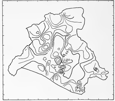
FIG. 4. Thickness contour of Berea Sandstone (feet), Lawrence County, Kentucky (from in-progress thesis by Morgan (10)).
