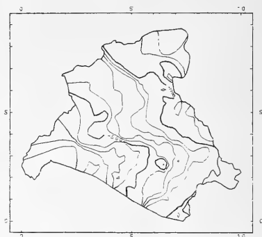
FIG. 5. Elevation contour of the top of the Berea Sandstone. (Contour interval = 100 feet.)
