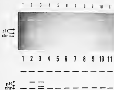
FIG. 1. Slab Gel Electrophoresis (1.0% agarose). Slots #1, #2, and #3 are control strains. Slot #1 contains strain 9440 which possesses only chromosomal (chr) DNA. Slots #2 and #3 contain MV154 and AC1, respectively and both possess chromosomal and plasmid (pl) DNA. Clinical isolates are located in slots 4-11 and reveal only chromosomal DNA.
