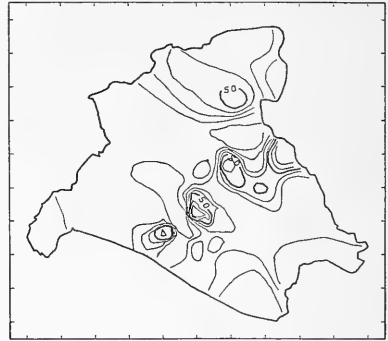
FIG. 9. Contour of sand per cent from cuttings number two, or second 20-foot interval, Lawrence County, Kentucky (from in-progress thesis by Morgan (10)).
