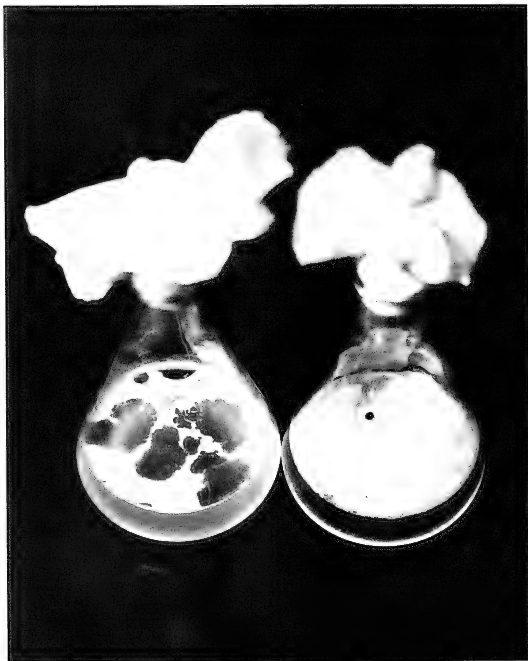
FIG. 5. Preliminary experiments showing zones of degradation occurring after 14 days of incubation at 25°C. Left: Flask inoculated with Acinetobacter calcoaceticus . Right: Uninoculated control flask.
