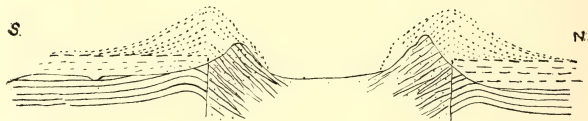
Plan and N-S section through Geitsi Gubib. In the plan the outline of the tuffs is indicated by the circular broken line; the broken line to the south is a path. A, B, C, D, E are satellite pipes; G, H, J, are tuff dykes. In the section the dotted lines show a reconstruction of the mountain as it may have been at the close of the outburst.
