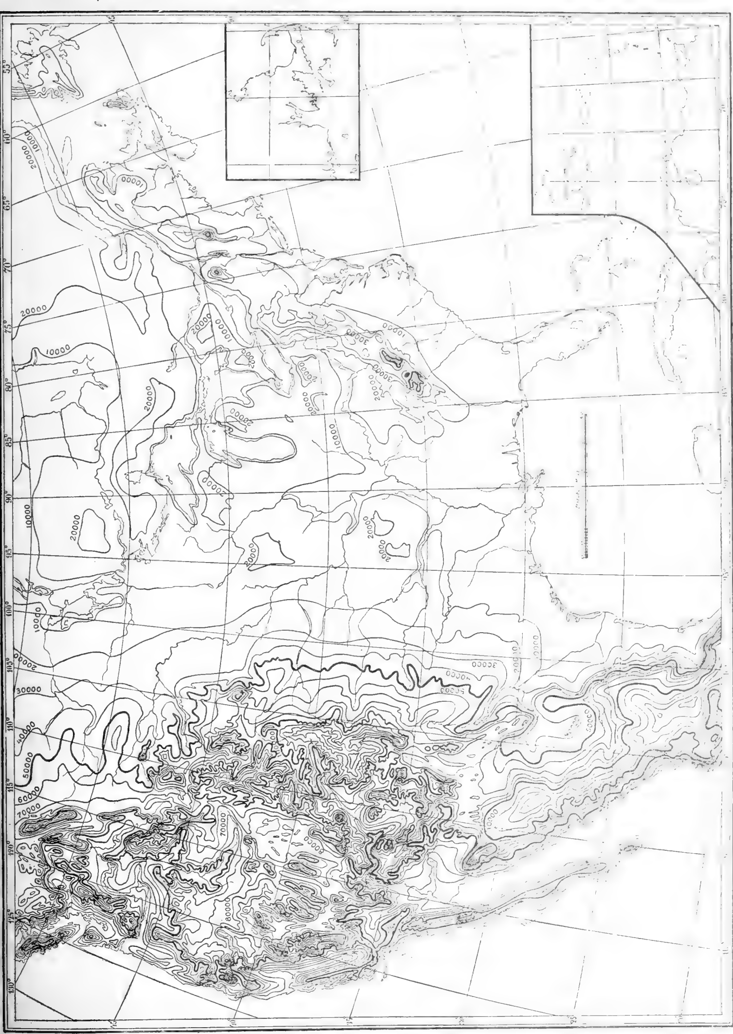
PLATE VIII. CONTINUED. LINES OF EQUAL POTENTIAL OF APPARENT GRAVITY AT THE SURFACE OF THE OCEAN.
