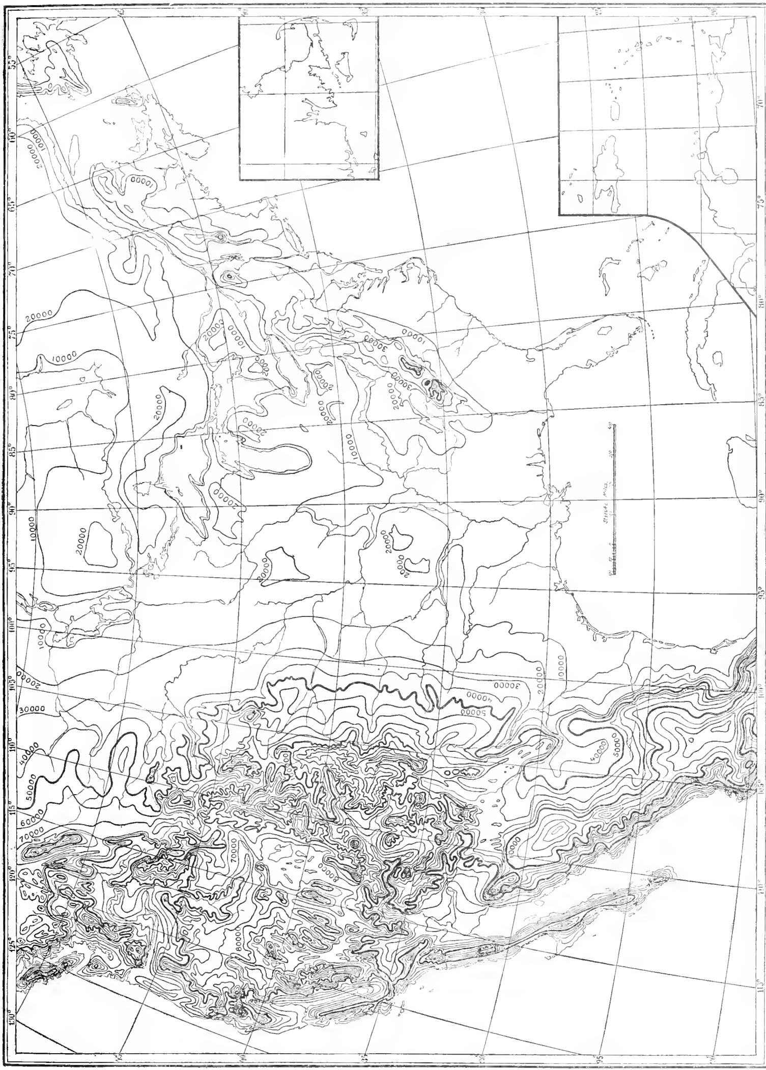
PLATE VIII. CHART OF LINES OF EQUAL POTENTIALS OF APPARENT GRAVITY AT THE SURFACE OF THE GROUND.
