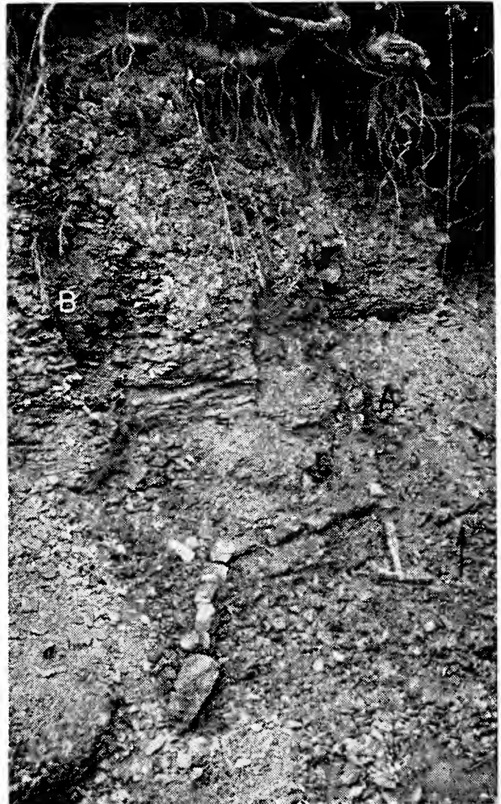
FIGURE 2.— Outcrop of shale with fissure fillings. Fissure fillings can be continuous for several feet (A) or may thicken and thin rapidly (B). Note hexagonal pattern.
