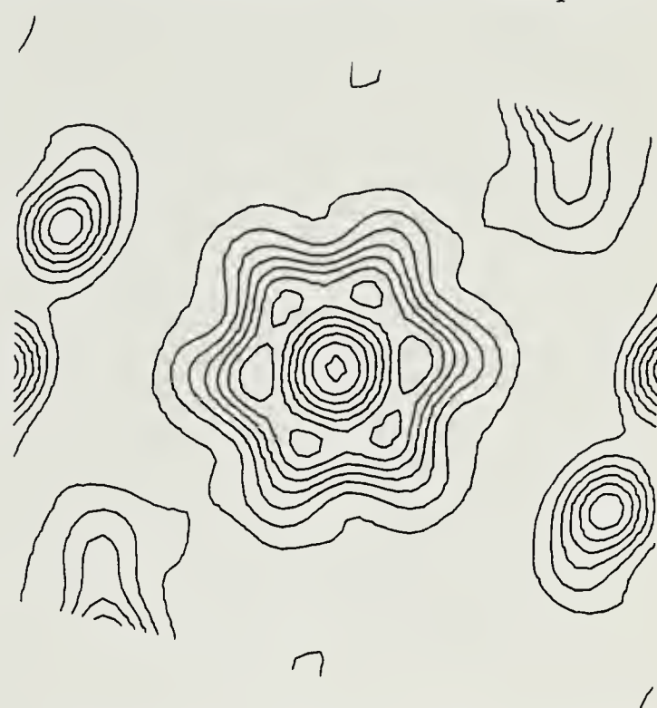
FIGURE 1c. Benzene outer electrons (1s isotropic state for carbon atoms has been subtracted). First contour line 0.2 \text{ e \AA}^{-3} .
