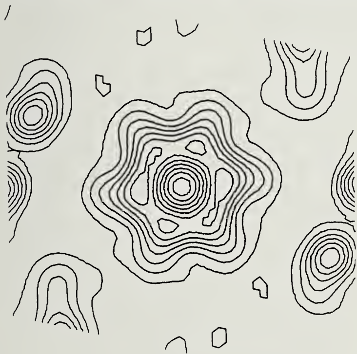
FIGURE 1b. Benzene outer electrons (a Gaussian core for carbon atoms has been subtracted). First contour line 0.2 \text{ e \AA}^{-3} .
