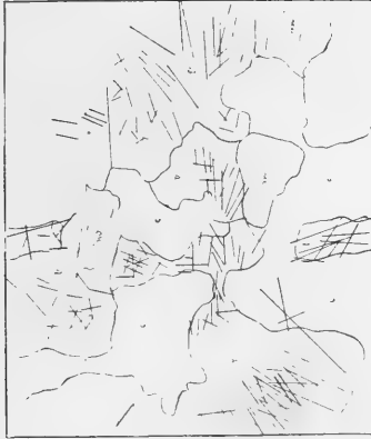
RUTILE NEEDLES IN QUARTZ, Q; CALCITE, C; BIOTITE, M.
