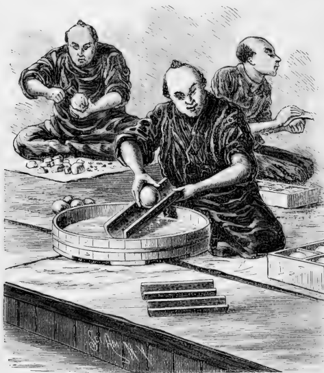
Japanese method of grinding and polishing crystal balls.
