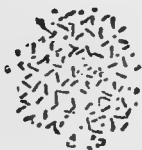
FIG. 4.—Acicular crystals in sapphire (enlarged 100 diameters).
