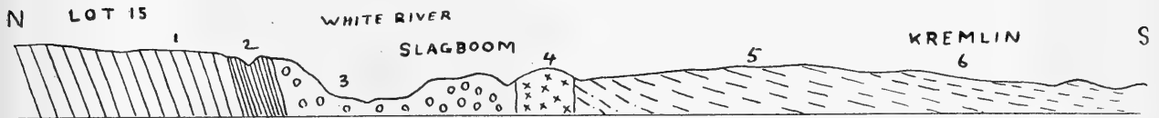
FIG. 3.—Section through Slag Boom, about 3½ miles. Vertical and horizontal scale the same. 1. Witteberg beds. 2. Lower Dwyka shales. 3. Dwyka conglomerate. 4. Volcanic rock. 5. Enon conglomerate. 6. Shales, &c., of Uitenhage beds.
