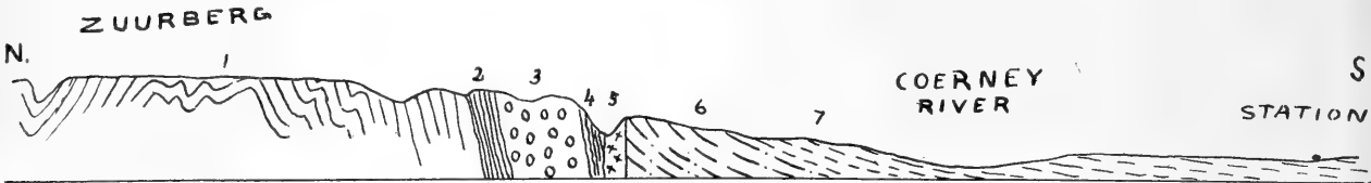
FIG. 1.—Section south from Zuurberg. Distance 8 miles. Vertical scale twice the horizontal. 1. Witteberg beds. 2. Lower Dwyka shales. 3. Dwyka conglomerate. 4. Upper Dwyka shales. 5. Volcanic rock. 6. Enon conglomerate. 7. Shales, &c., of Uitenhage beds.
