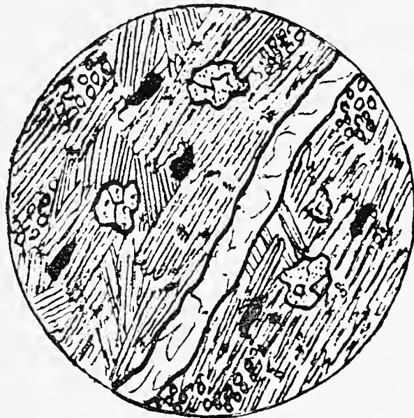
Fig. II. Microscopic Section of Banded Hornblende Schist from Balhoulan Quarry. X 50 Diameters.
