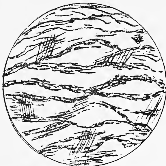
Fig. III. Microscopic Section of Grit Band in Hornblende Schist from Balhoulan Quarry. X 50 Diameters.
