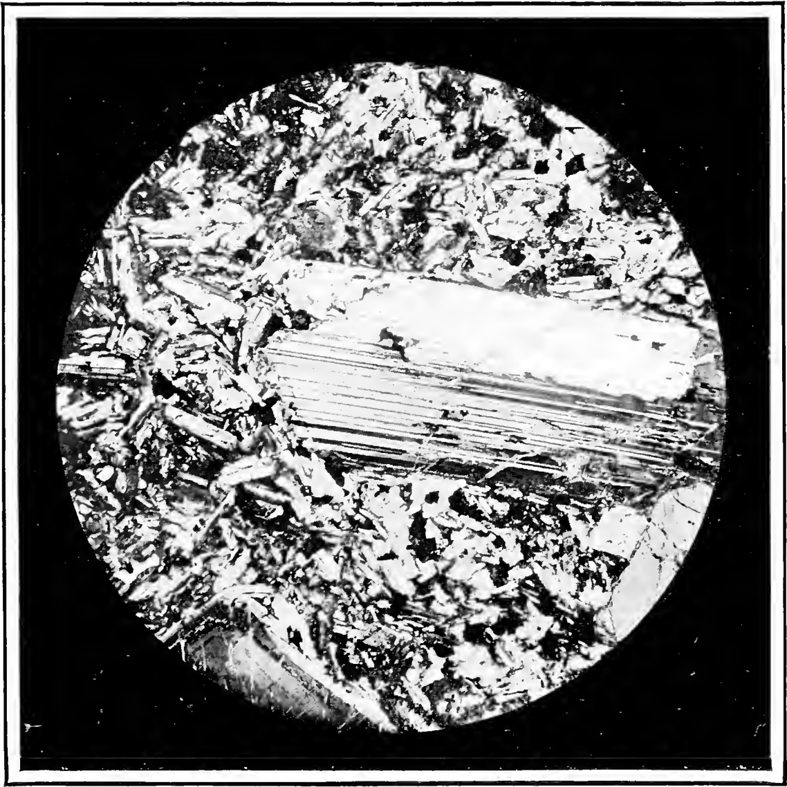
Plate 42.—Felspar Phenocryst viewed by Polarised Light, Andesite, Muirhall, x 36.
