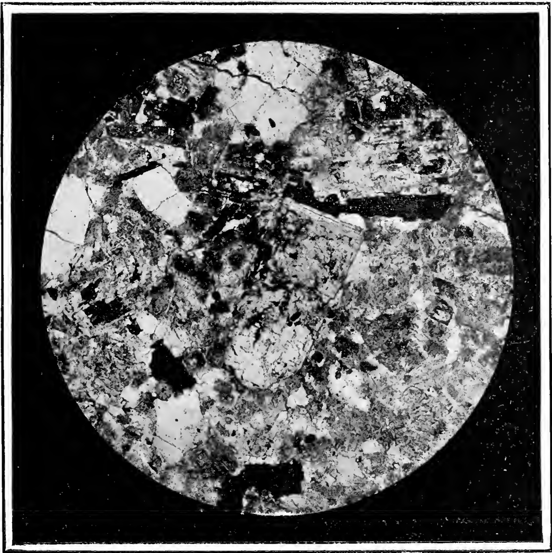
Plate 55.—Biotite-Granite, Glen Lednock, magnified 10 diameters.
