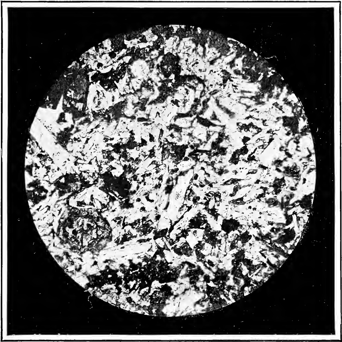
Plate 41.—Corsiehill Andesite, Ground Mass, x 50.
