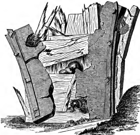
4\frac{1}{2} -in. plate, faced with 4-in. rubber, after three 11-inch shot.
