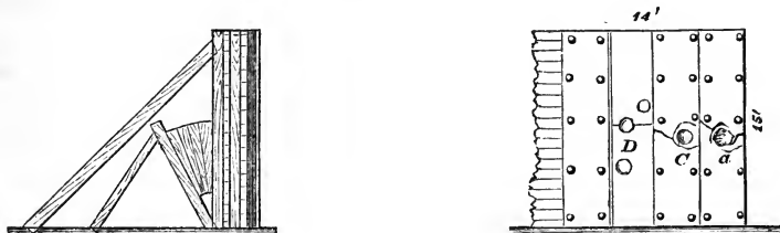
Side and front of 6½-in. laminated target.
