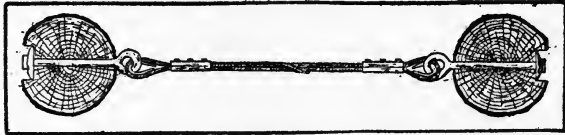
Method of attaching eyebolt and stranded wire.
