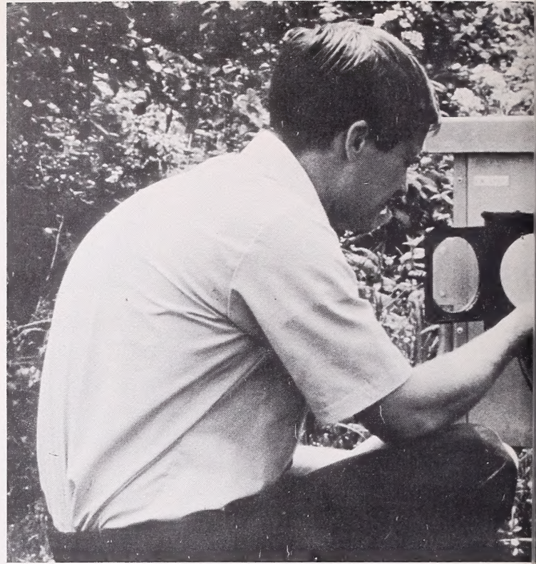
An air pollution sampling device is checked. Air is drawn through a filter that catches particulates, and thus provides data for the force to evaluate.
