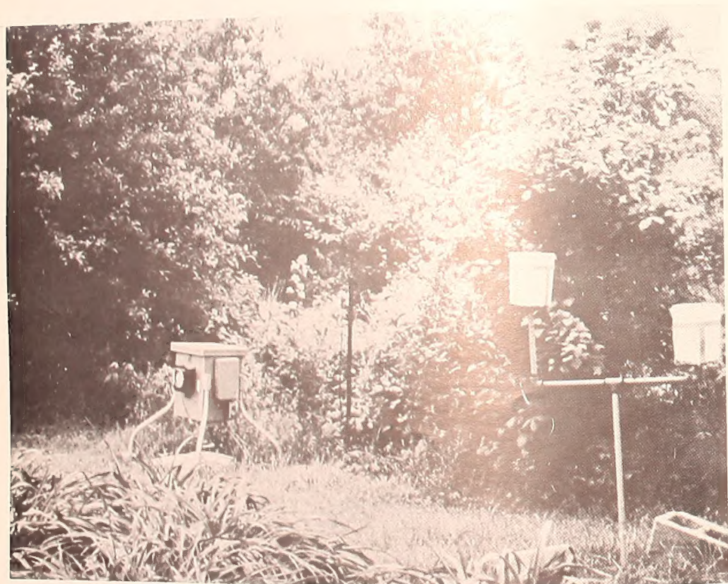
Aerial sampling for particulate pollutants is done with the dustfall bucket (lower right) for larger sizes of settling pollutants and with a Hi-Vol sampler for smaller particles, which tend to remain air-borne for indefinite periods. This set-up helps measure dustfall and suspended particles in an open area.
