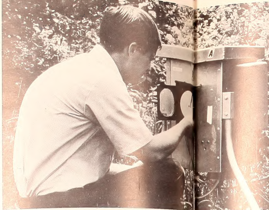
An air pollution sampling device is checked for accuracy. Air is drawn through a filter that catches the particulates, and thus provides data for the forestry researchers to evaluate.
