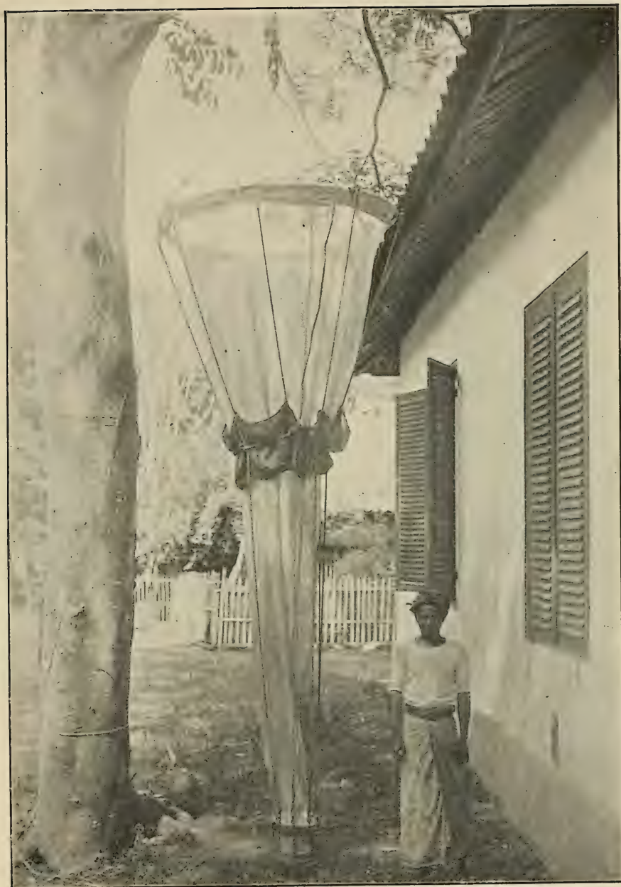
Larger vertical closing net, open. Length of the net 4 M., diameter at the entrance 1,3 M., silk gauze no. 3.
