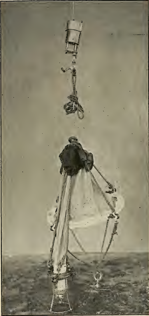
Smaller vertical closing net, closed. Length of the net 1,5 M., diameter at the entrance 0,5 M., silk gauze no. 25. The line connecting the closing mechanism and the net has been coiled up.
