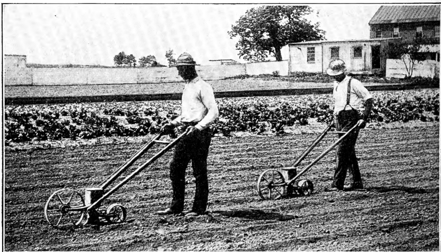
Plate III. A modern American hand drill planting onion seed. Modern drills plant seed any depth, any distance apart, in rows or in hills.
