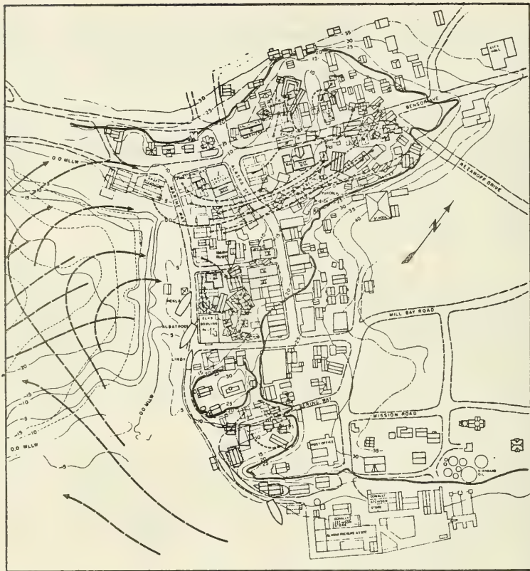
Figure 49. 1964 tsunami runup, Kodiak City, Alaska (contours in feet); heavy line is maximum flood level (from Wilson and Tørum, 1968).
