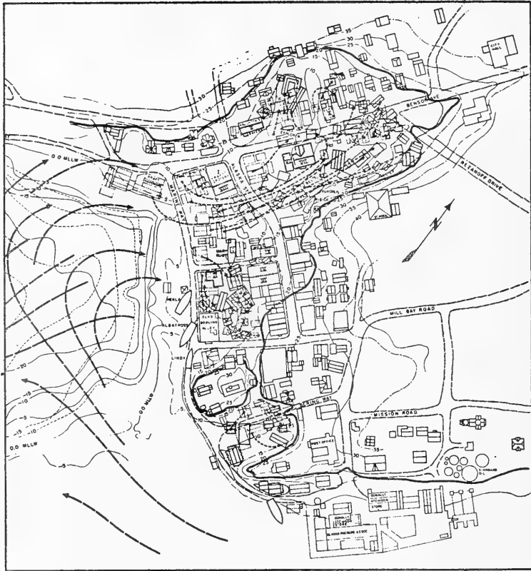
Figure 49. 1964 tsunami runup, Kodiak City, Alaska (contours in feet); heavy line is maximum flood level (from Wilson and Torum, 1968).
