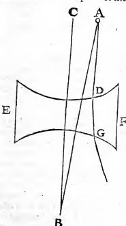
And taking a body of concave furfaces we shall (according to this doetrine of ours ) find the causes of refraction just contrary; & accordingly experience likewise sheweth us the effects to be fo too. And therefore fince experience agreeth exactly with our rules, we cannot doubt but that the principles upon which we go are well laid.
