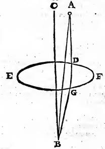
be a Lens or a glaffe on both fides convex; and CB the axis of it; AD the ray falling from the illuminant A; AB the perpendicular falling fro the same illuminant A:it will be plain by the former discourse, that the ray A D, must at the entry be refracted towards AB, as being repulsed from that part of the infide of the pore D, which is towards F; because that fide is most opposed unto the ray. Now the ray being once turned way; when at the end of its journey through the glaffe
