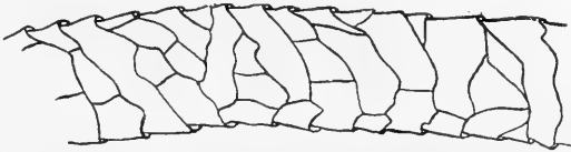
Fig. 80. Wool Fiber Highly Magnified.
