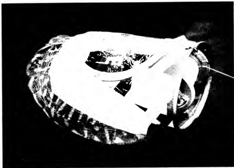
FIG. 1. Thread-laying device ("trailer") taped to the carapace of an adult female T. o. ornata . The squares of tape on the sides are to keep the bent-over ends of the wire axle from catching on vegetation ( \times \frac{1}{2} ).
