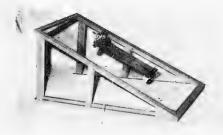
Fig. 12 - Device having four rubber-covered heels and weighing 1275 grams, climbing a sheet of glass inclined at  $59^{\circ}$
