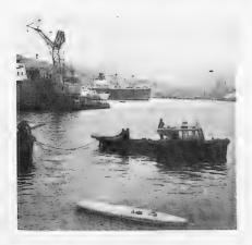
Fig. 18 - Hull of float in Fig. 17, showing the wave produced by its lateral displacements
