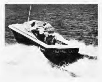
Fig. 10 - The planing craft Thunderbird propelled by the Pratt and Whitney Sea Jet-6 waterjet system
