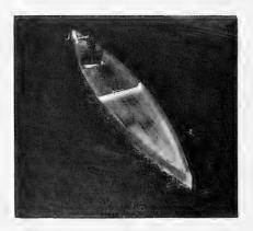
Fig. 19 - Very light hull, 1.40 meters long, flat bottom, driven by a device with two masses
