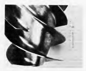
Fig. 9 - High-solidity rotor used in the Pratt and Whitney waterjet system Sea Jet-6
