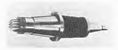
Fig. 7 - Six-component balance
