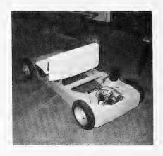
Fig. 14 - Device on back part of a wooden frame set on four automobile wheels, consisting of two masses of 3 kg each. The masses are put in motion by a 12-volt automobile battery and move the back part of the frame sideways, in the direction of rotation
