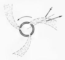
Fig. 5 - Radial-flow cryptosteady pressure exchanger
