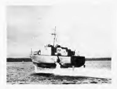
Fig. 7 - The waterjet-propelled hydrofoil craft Tucumcari (designed and constructed by the Boeing Company for the U.S. Navy)
