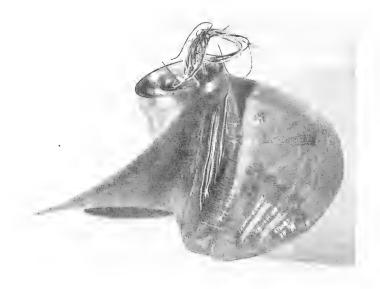
Fig. 31 - Strain-gauged hydroelastic propeller
