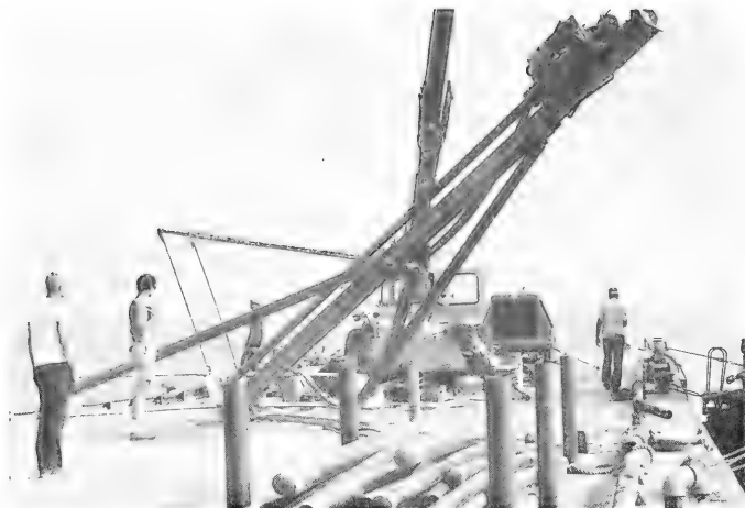
Figure 2. Vibratory core rig with a 20-foot-long barrel used in a geological survey in Lake Erie. An articulated leg is used to allow the rig to be placed on the platform deck for insertion and removal of the core liner. Note recovered cores contained in the crib area in the foreground.
