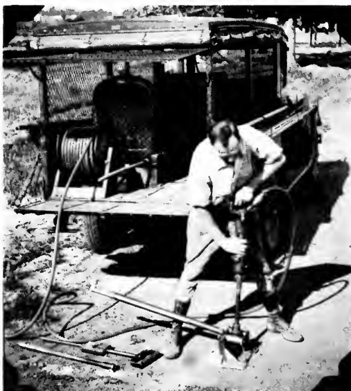
B. Soil sampling equipment: compressor unit (on truck), pneumatic driving hammer (in operator's hands), ordinary soil tube hammer (on ground) and soil tube jack.
