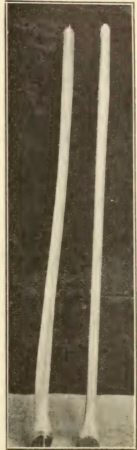
FIG. 7.—Blue-gum (crooked) and hickory (straight) ax helves. Blue-gum helve cut from plank air-seasoned for two years.
