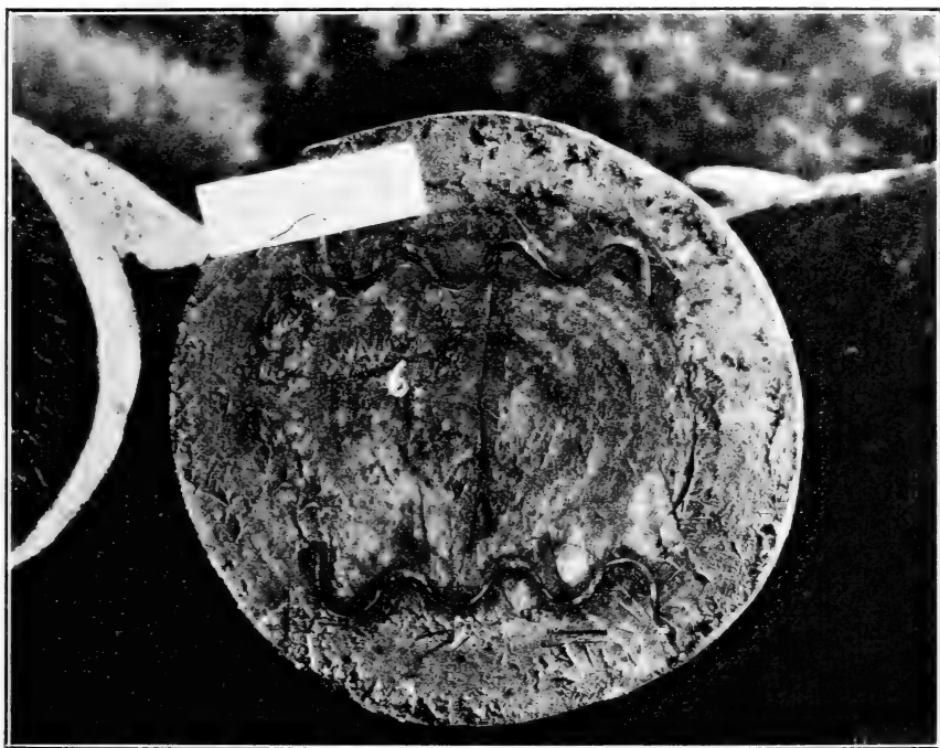
FIG. 5.—Blue-gum log protected with S irons to minimize checking during seasoning.
