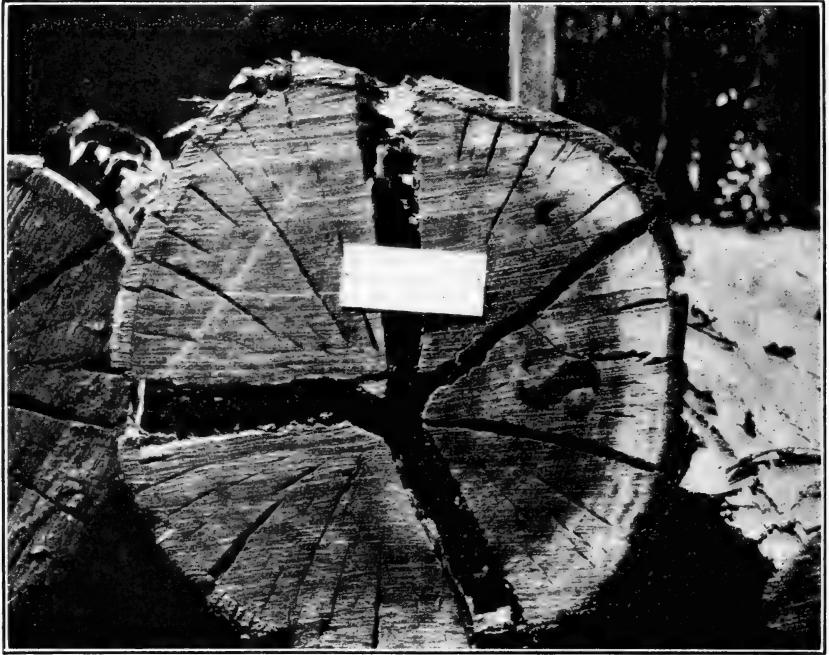
FIG. 4.—Unpeeled blue-gum pole cut March 26, after four months air seasoning. Sutro Forest, San Francisco, Cal.
