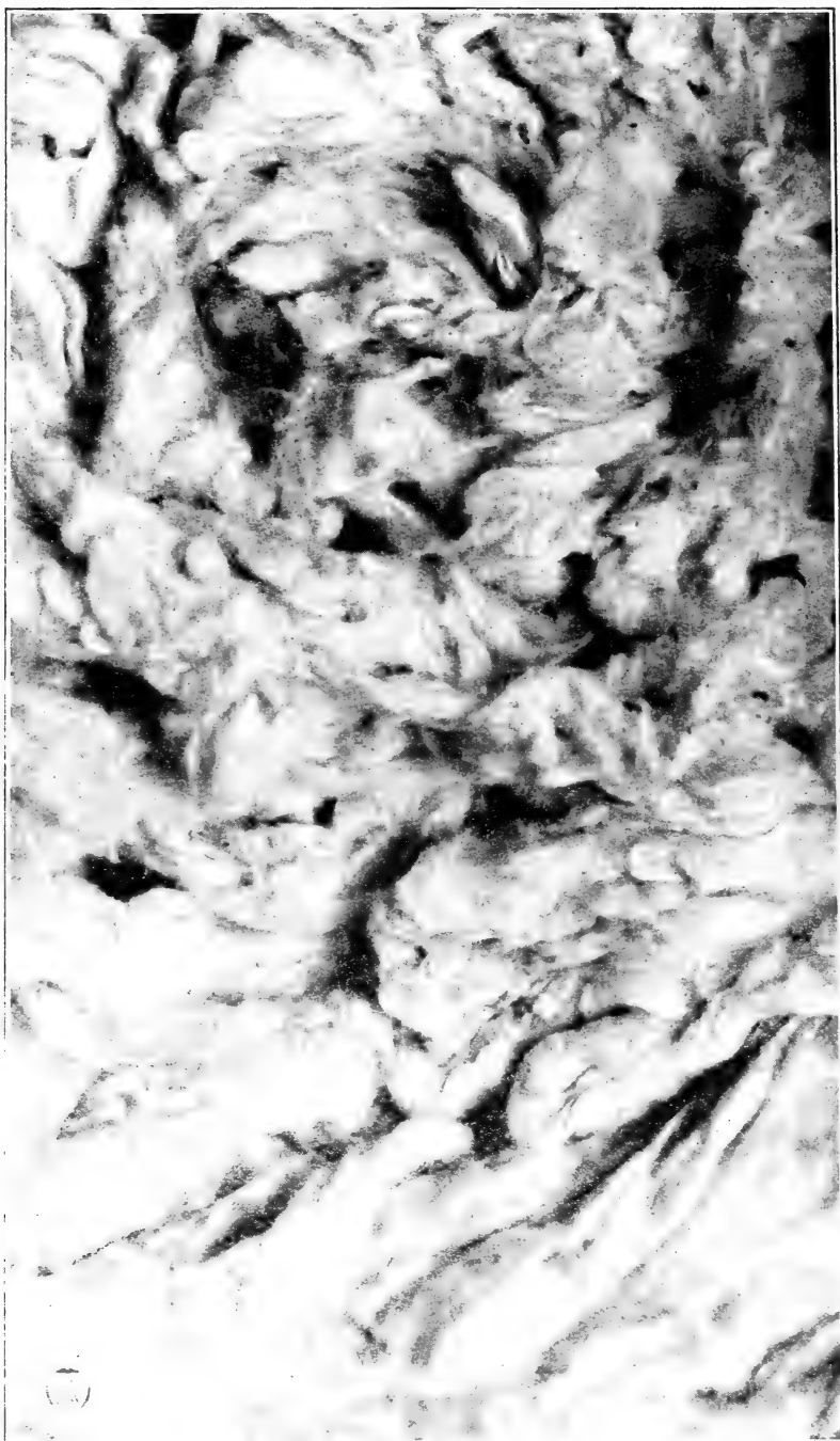
COTTON SAMPLE SHOWING CURL, FLOCK, AND CUT SEED.
