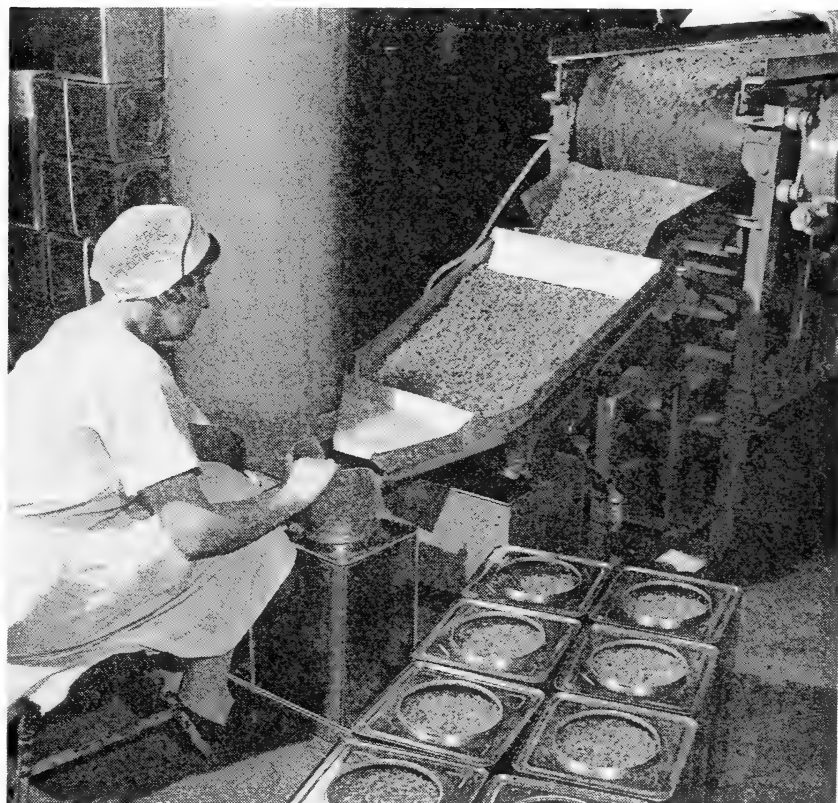
FIGURE 61.—Filling 5-gallon cans with diced dehydrated carrots.
