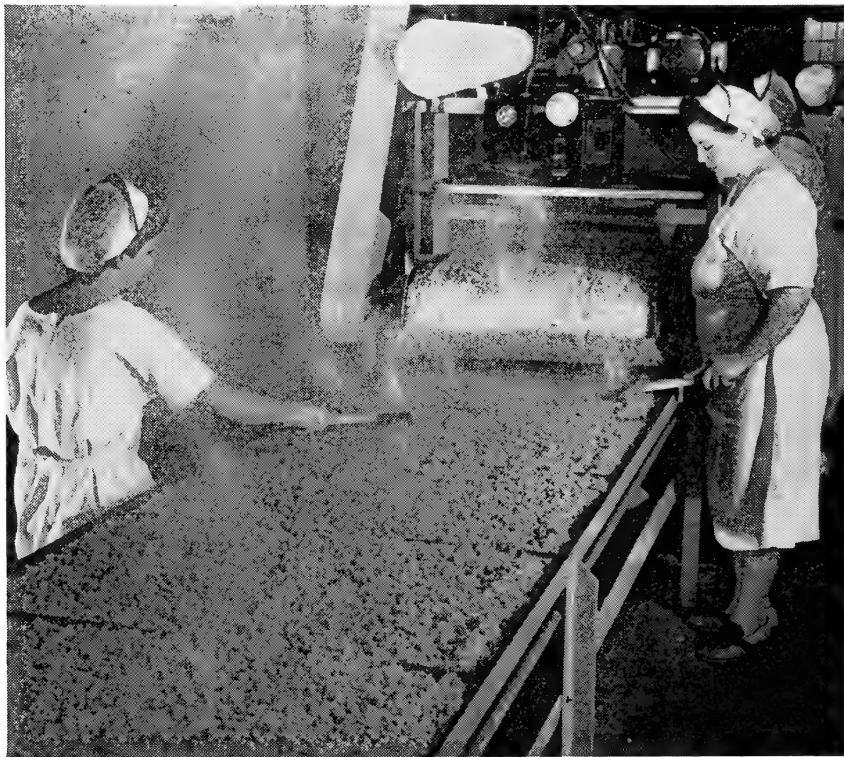
FIGURE 21.—Steam-blanching diced carrots being loaded directly from the blancher on drying trays.
