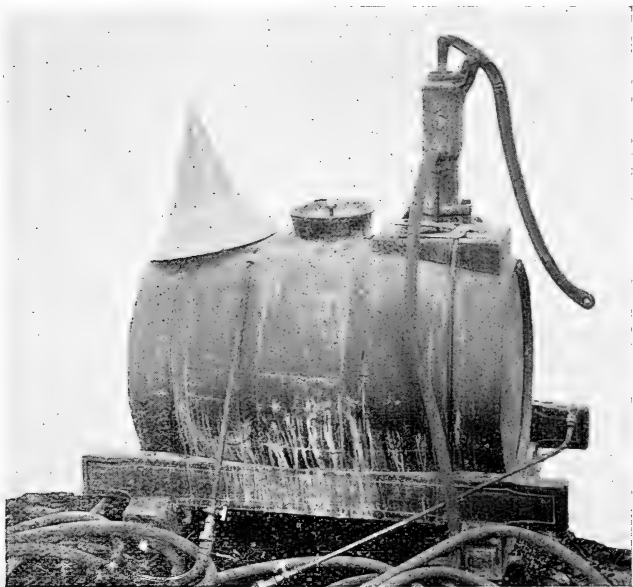
Figure 14.—Barrel spray pump. showing cone shaped strainer to the left. frame and may be placed in a wagon or on a stone boat when it is to be used.
