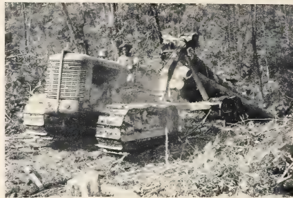
FIGURE 37.—Tractors are used by larger mills to skid logs to road or railroad.
