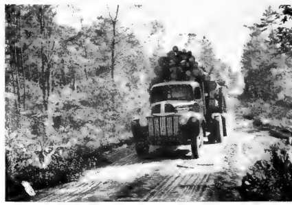
FIGURE 38.—Trucks are being used increasingly to get logs to the mill. Note metal airfield landing mats on roadway.
