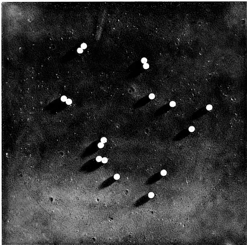
FIG. 8. A drop-pattern of poliomyelitis virus. \times 12,000 . The large spheres are polystyrene latex particles that have been mixed with the virus at a concentration of 3.2 \times 10^{10} particles/ml. From the number of these particles and of the poliovirus particles in this drop pattern it can be concluded that the virus was sprayed at a concentration of 3.8 \times 10^{11} particles/ml.
