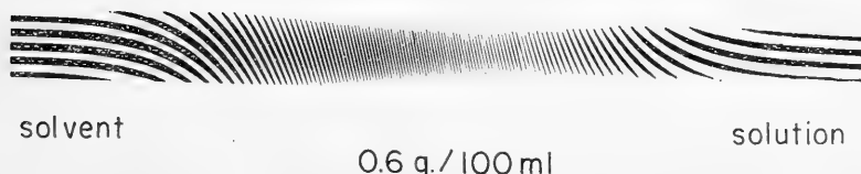
FIG. 2. Representative Rayleigh interference patterns obtained during the diffusion of bushy stunt virus. (From Cheng and Schachman, unpublished.)
