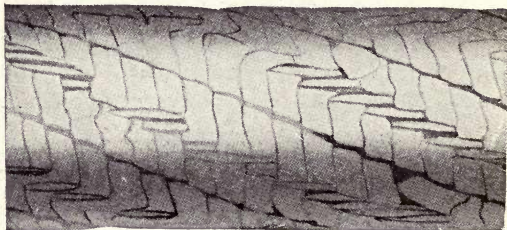
Side view of worn rope.
