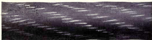
Cut showing Waterbury Fibreclad Rope after constant service and after covering has worn to the strands
