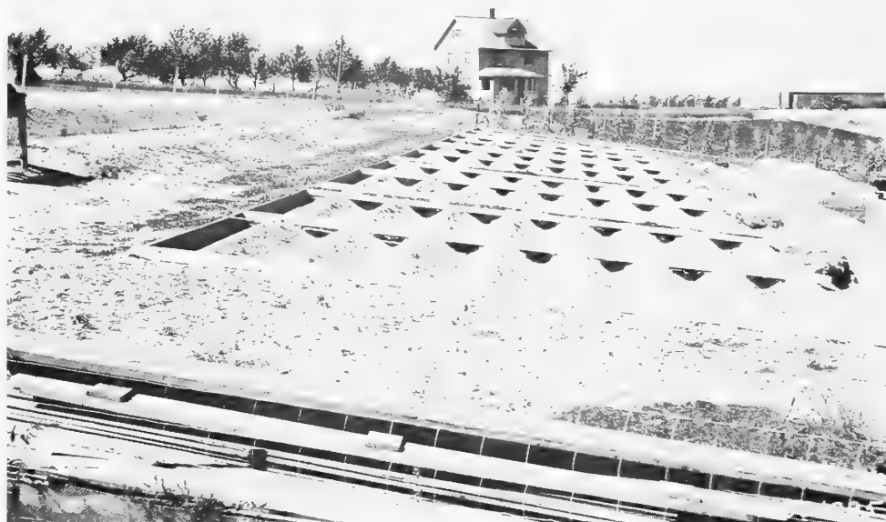
F-331095 FIGURE 3. — Completed lysimeters before treatment. The terraces were built to prevent runoff and soil loss during the first year of seedling growth, and to test the uniformity of percolation. The lysimeters have a 10-percent slope to the right.
