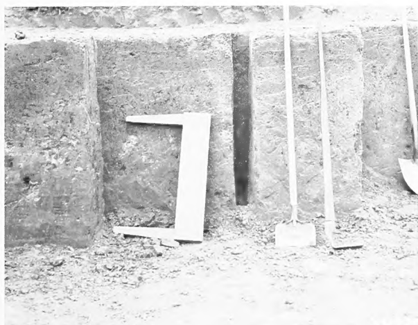
F-331079 FIGURE 2. — How soil blocks of loess were cut from a natural profile.
