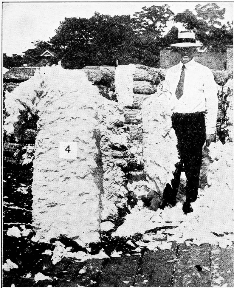
FIG. 4.—Bale No. 4 (test No. 2) during the process of "picking" or reconditioning. Only a portion of the damaged cotton has been removed so as to show the depth of the damage. (The damaged cotton is compact, while the cotton not damaged is fluffy.) This bale lost 209 pounds, or over 43 per cent of its gross weight as a result of the exposure (See Table 2)
