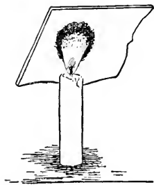
C.—THE CARBON (OR SOOT) IS DEPOSITED ON THE GLASS.
