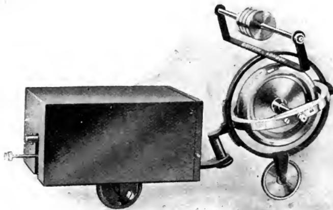
Gyrostatic Motor Car with two wheels in tandem. The car can be set to run in a straight path, or in a circular path in either direction.
